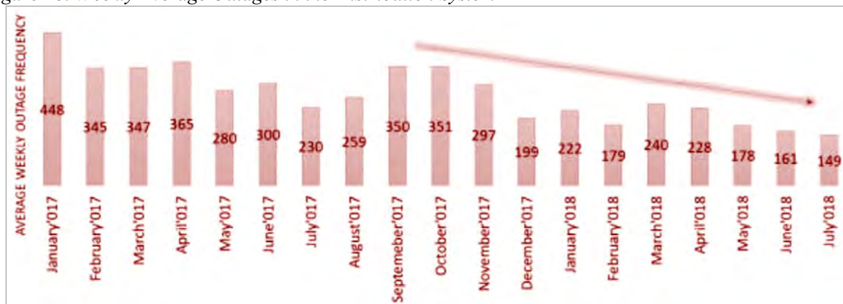
Figure 18: Weekly Average Outages in the Distribution System
