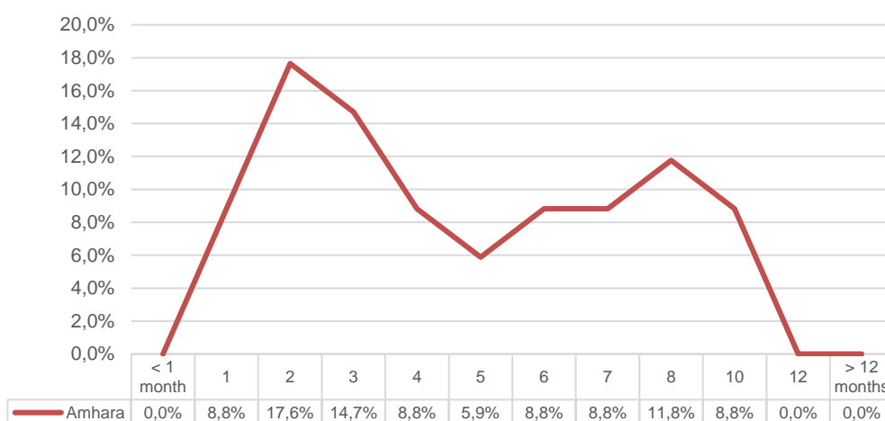
Figure 19 - Distribution of non-functional bio-digesters by number of months
