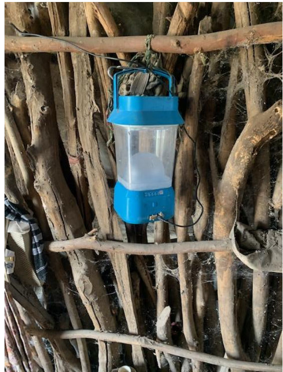
Exhibit 14. Solar Lanterns are provided as replacement to biogas lighting to protect grass hut homes against fire. Afar Region
