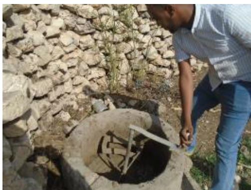
Figure 78 - Dung mixer locally manufactured in Somali region used in Owbarre Woreda.
