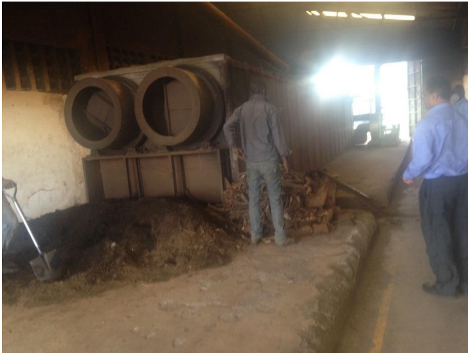
Figure D2: Sawdust dryer at the factory. The dryer runs on biomass feed, mostly twigs and left-overs from lumbering activities
