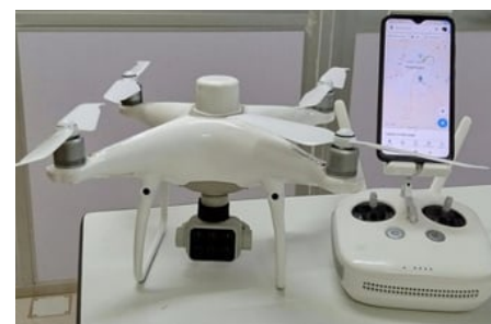
Phantom 4 multispectral drone optimised for digital mapping in agriculture Burkina Faso (WASCAL, 2021)
